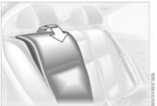
The backrest moves forward slightly when released. Reach into the gap and fold it down.
